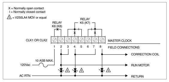
Figure B-22 Stromberg Synchronous Wired (56th Minute)
